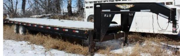
\* 04' H&H 30' flatbed w. 3 pc. HD ramp system. Tandem singles w/ 14K axels. Good floor, lights & breaks & twin jacks
